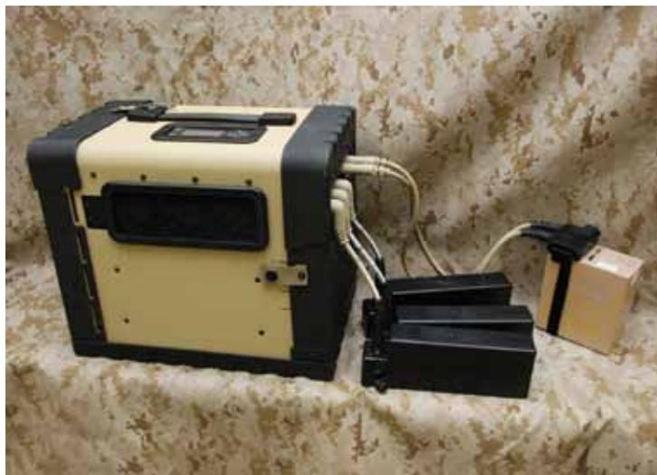
A 300-WATT FUEL CELL USED BY THE ARMY. FUEL CELLS ARE ESTIMATED TO BE 83% MORE EFFICIENT THAN TRADITIONAL GENERATORS.
