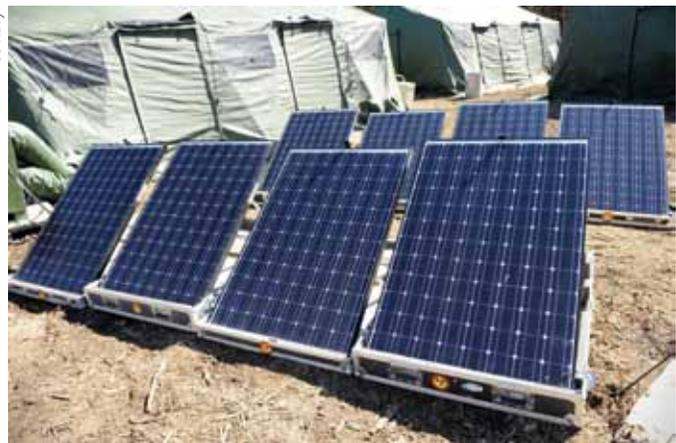
**US NAVY-WATT PHOTOVOLTAIC BATTERY SYSTEM, DEVELOPED BY THE OFFICE OF NAVAL RESEARCH, CAN PROVIDE CONTINUOUS POWER TO MARINES IN THE FIELD**
