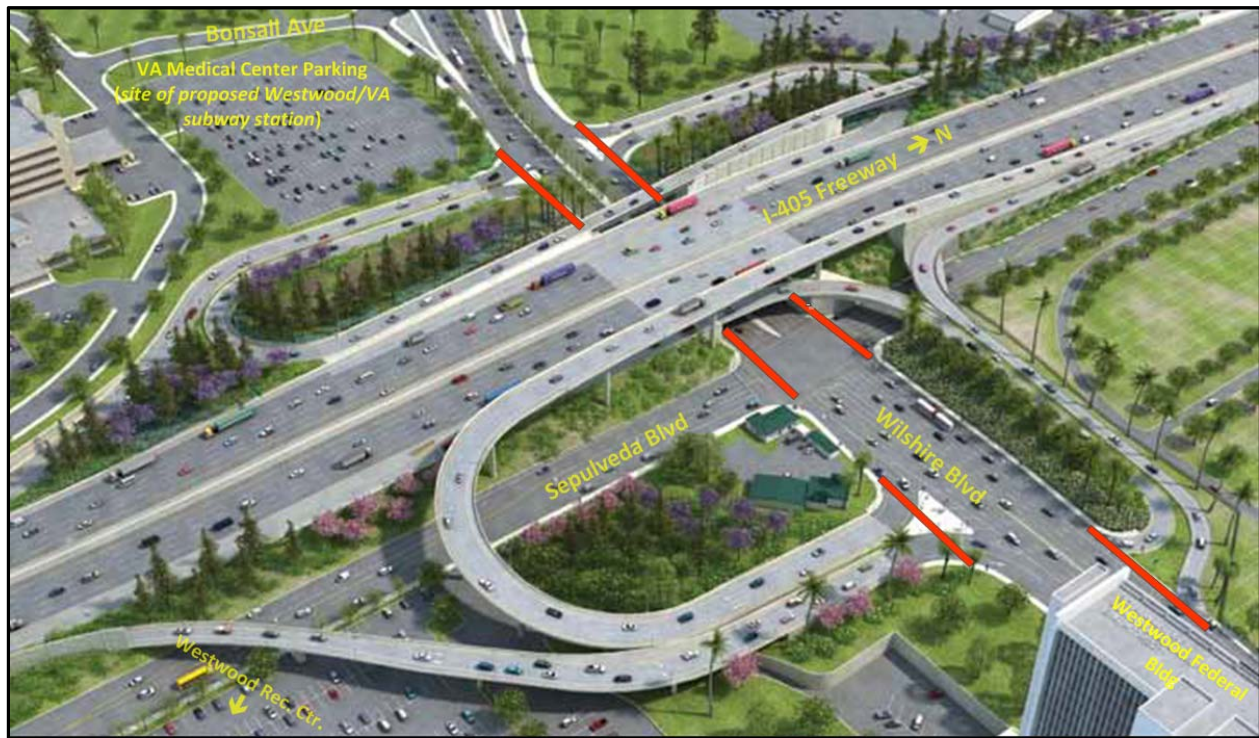
Figure 8: Intersection of Wilshire and Sepulveda Boulevards and I-405 Freeway interchange with red lines indicating areas where high speed vehicle traffic, freeway off-/on-ramps and tunnels create hazardous conditions for bicyclists and pedestrians traveling along Wilshire Boulevard. Non-annotated graphic courtesy Metro. Annotations added.
