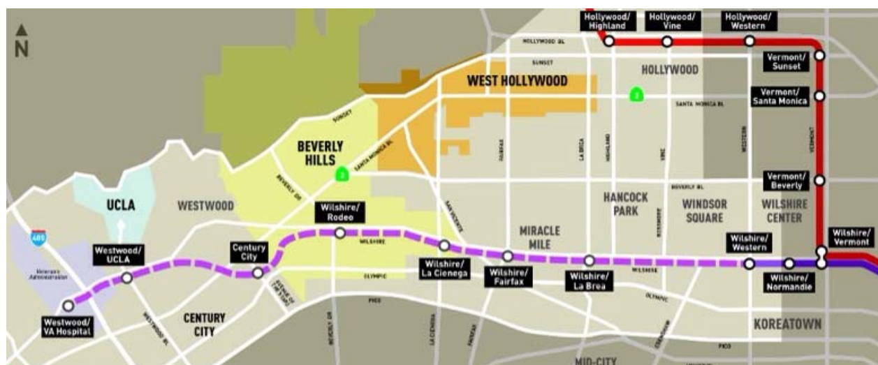
Figure 1: Wilshire Corridor, Mid-City and Hollywood areas of Los Angeles showing current Metro subway lines (solid red and purple lines) and the proposed Westside Subway Extension (dashed purple line). For most of its proposed route the Westside Subway Extension would follow the Wilshire Corridor, except for a brief section from the western edge of Beverly Hills to Westwood where it dips south to Century City. (Map courtesy of Metro)
