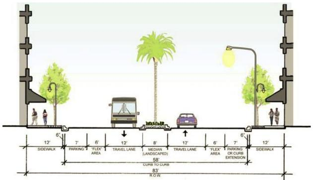
Figure 7. Cross-section view of the recommendation for Mission Street between Silver Avenue and Rolph Street (SFCTA 2007)
