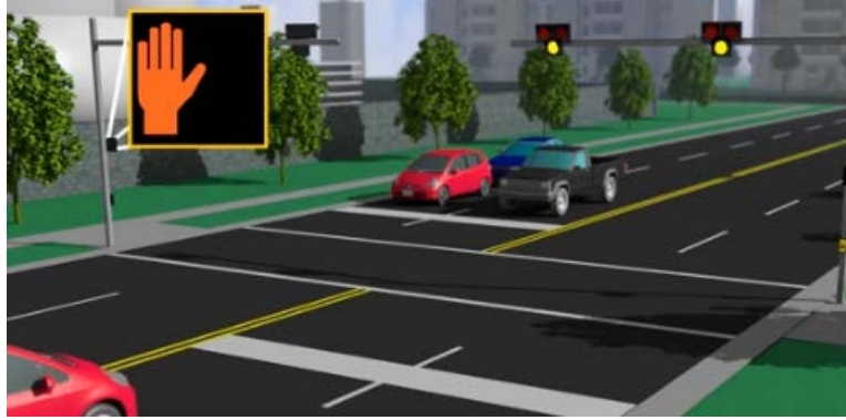
Figure 28: Pedestrian Hybrid Beacon - Installation on State Route 25 Source: Chatham County Department of Engineering
