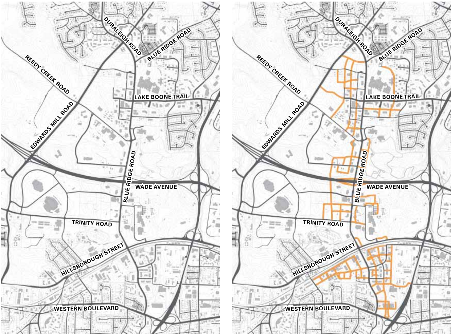
Figure 5. An excerpt from the BRR small area plan, showing the current road network (left) and the proposed network of secondary streets (right, in orange) to increase connectivity between destinations within the corridor. All new and repaved streets would include sidewalks and bicycle facilities. 16
