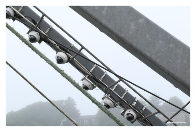
Fixed lens cameras affixed to the forward rigging of a bottom trawler.
