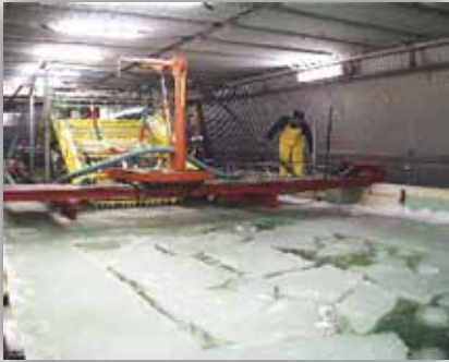
Figure 5-12. Example of Tank Test for Mechanical Recovery of Oil Spilled in Sea Ice (Photo: Nuka Research)—During wave tank tests, ice is typically frozen under controlled conditions to the desired thickness and concentration, and various technologies are tested. The ice is then combined with oil in tanks of various sizes to test equipment. At left, ice was created in tanks at the U.S. Army Cold Regions Research and Engineering Laboratory and used in a series of skimmer tests.
