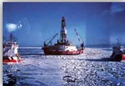
Figure 3-6. The Kulluk Drill Ship —The Kulluk, built in 1983, was the first floating drilling unit constructed for Arctic waters. The Kulluk drilled 12 wells in the U.S. and Canadian Arctic Ocean in the 1980s and 1990s. The Kulluk was purchased by Shell in 2005 and refurbished to support planned OCS drilling in the U.S. Arctic Ocean beginning in 2010. A major alteration of the Kulluk was the addition of thrusters, changing the drill ship from a barge that required towing to a self-propelled vessel.
