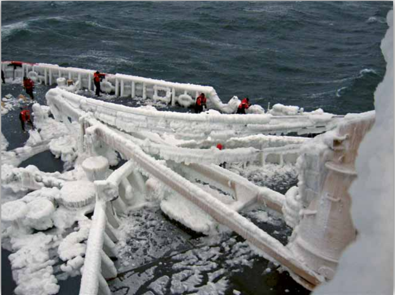
Figure 6-1. Ice Obstacles (Photo: USCG)—Ice can form on vessels, making it more difficult to operate machinery and equipment.
