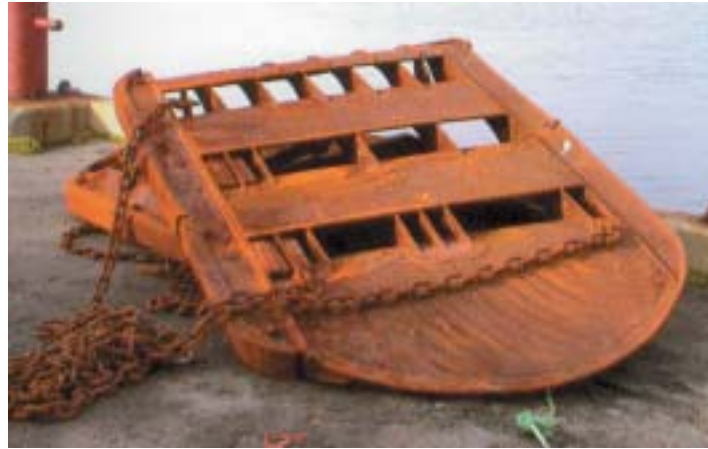
Two trawl doors and chain can weigh 10 tons.
