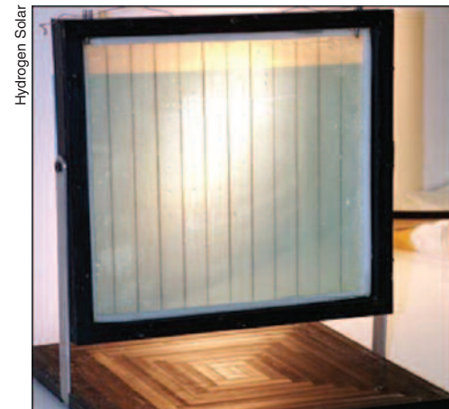
Hydrogen Solar's Tandem Cell uses sunlight to split water into hydrogen—potentially a clean source of fuel—and oxygen. The cells have nanocrystalline metal particles on their surface, giving them a vast area with which to collect the sun's energy.
