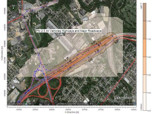
Figure 10: PM<sub>2.5</sub> Emissions from Existing Vehicle Volumes
