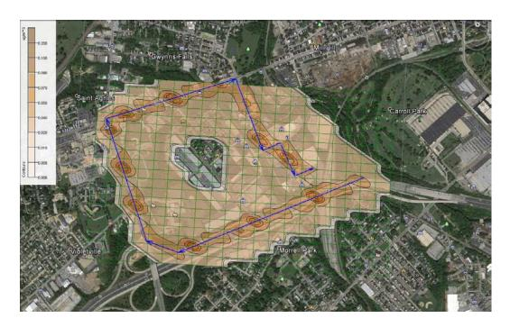
Figure 14: Impact of Truck Traffic Increases on  $PM_{2.5}$  Emissions along Bernard Drive Route (assuming the trips are evenly spread)
