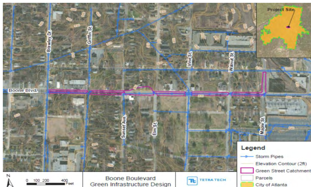
Figure 20. Map of underground storm pipes around the proposed project site. (Source: Tetra Tech 2013)
