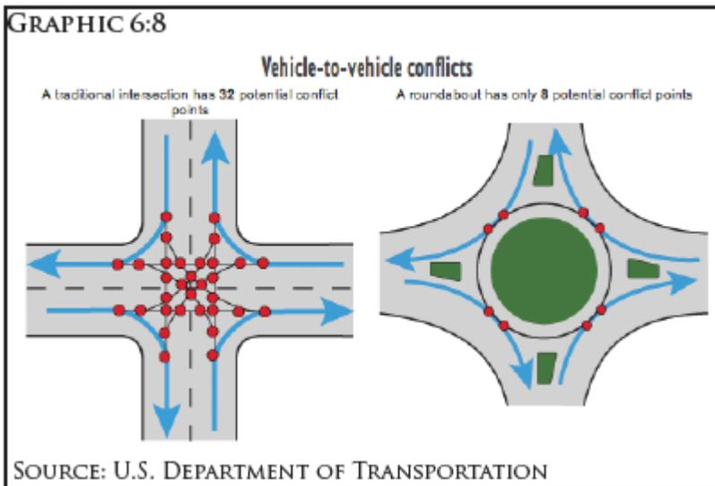
As can be seen in Graphic 6:8, roundabouts limit the nodes-of-impact that are created by normal intersections. Roundabouts improve navigation by providing an easy, safe location for U-turns, an action that is increased when seeking parking or an event location.
