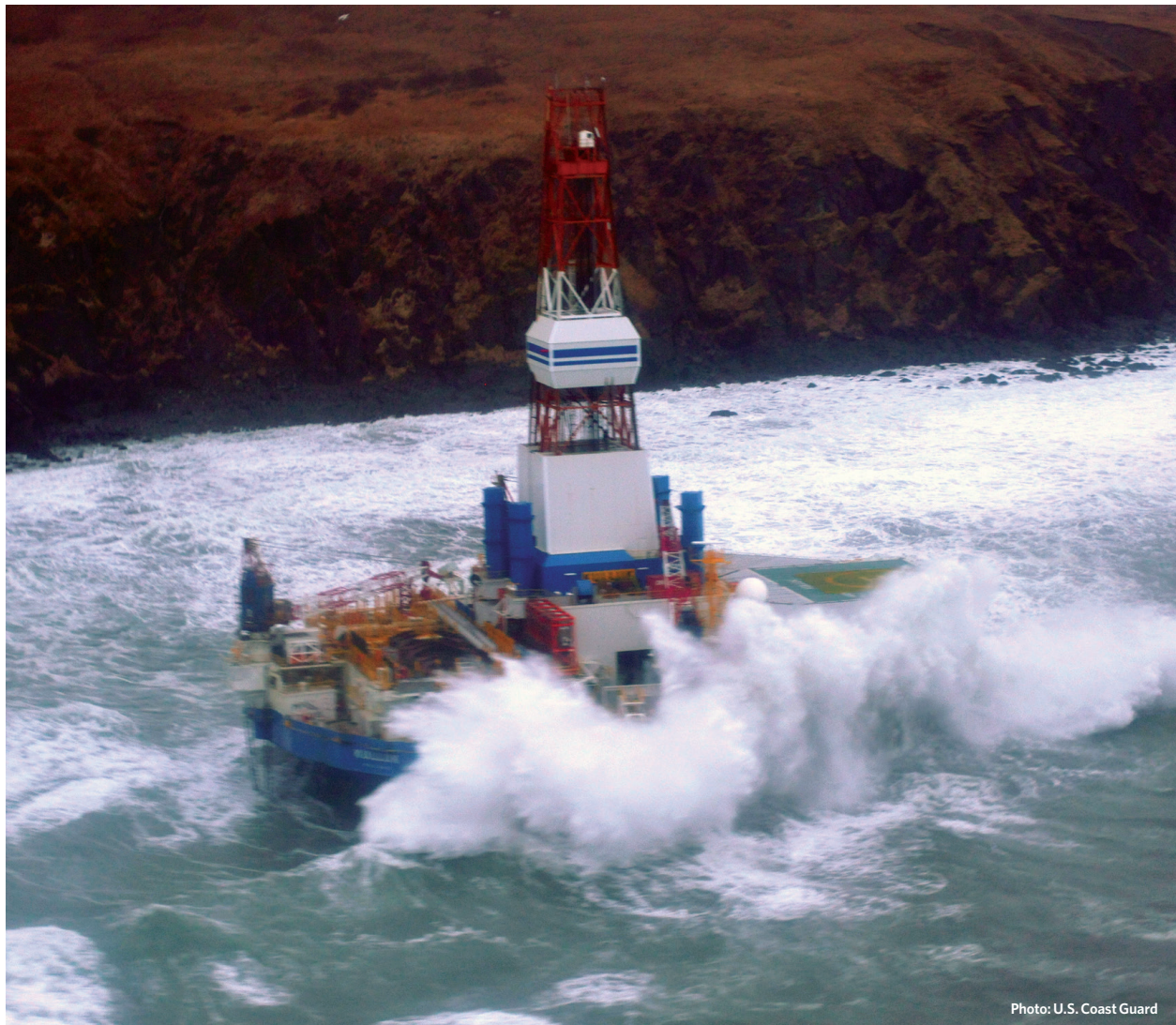
A Shell Oil drilling rig, the Kulluk, ran aground in late 2012 after towlines broke and the vessel towing it suffered multiple engine failures.
