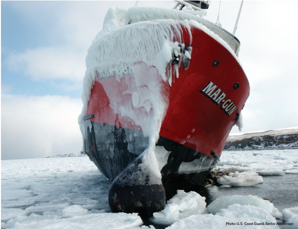
Fishing vessel Mar-Gun grounded on St. George Island in the Bering Sea. Ice accumulated on its starboard side. Freezing temperatures and sea spray can also create structural icing during transit that can be dangerous for a vessel's stability and crew safety.
