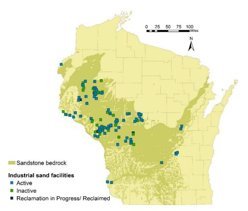
Figure 1.1. Industrial sand mines and processing facilities as of September 2015. Sandstone bedrock extent represents the rock type generally targeted for industrial sand mining. Sources: Wisconsin Department of Natural Resources and Wisconsin Geological and Natural History.
