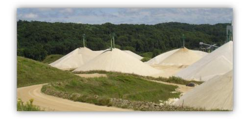
Washed silica sand, stored in piles before drying and shipment. Courtesy Badger Mining Corporation.
