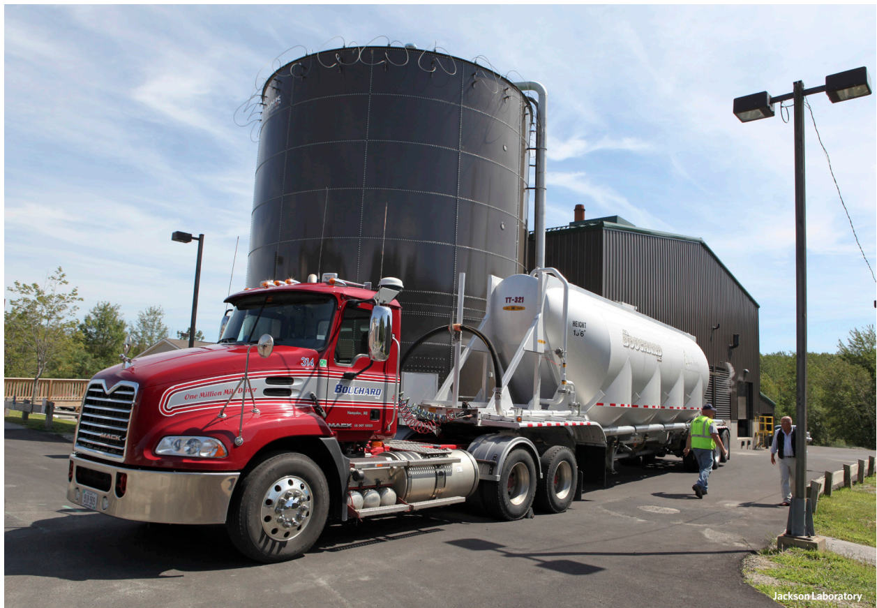
Truck unloading wood pellets for a biomass combined heat and power plant at the Jackson Laboratory in Bar Harbor.
