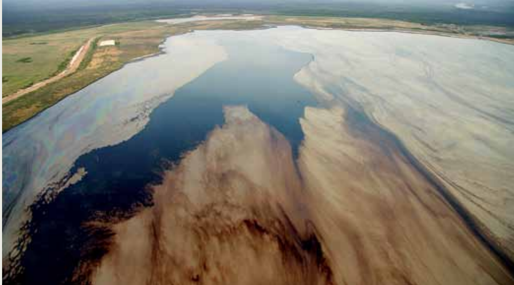
Toxic liquid byproducts created during the upgrading process are often pumped into large, open tailings ponds.
